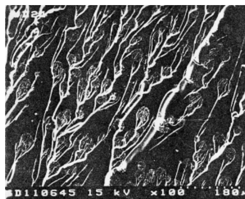
Figure 8 SEM observed impact fracture surface of polyester/epoxy resin blends prepared in the normal gravity.
