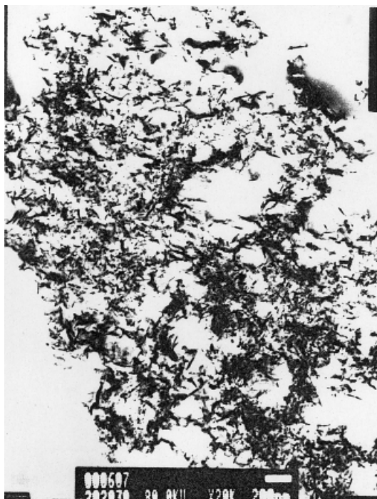
Figure 9 TEM micrograph of PET/EP blends prepared by an acoustic levitation.
